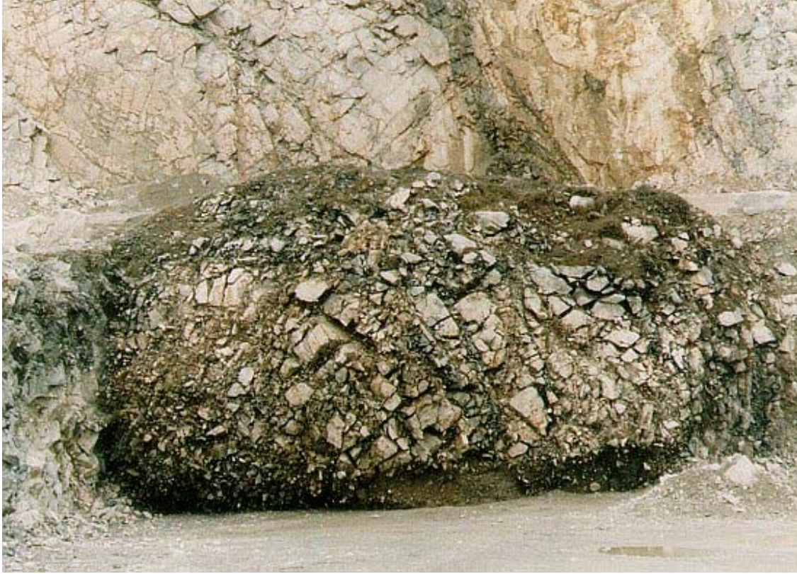
Figure 4. A normal, well-controlled blast in progress with similar charge design to that proposed at new Shine, in which no forceful rock projections occur from any part of the blast.
